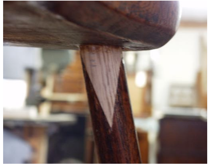
fig.2 A double-wedge splice on one stanchion for a cheval mirror and a splice to a Windsor chair leg.
