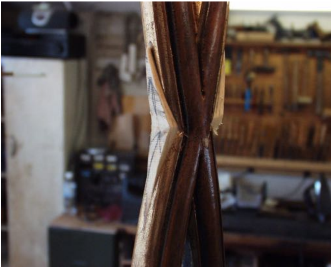
fig.2 A double-wedge splice on one stanchion for a cheval mirror and a splice to a Windsor chair leg.
