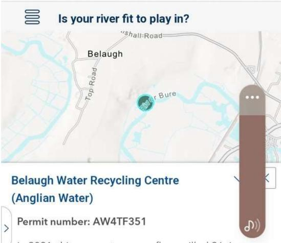
In 2021, this sewer storm overflow spilled 96 times for a total of 1749 hours, discharging into the River Bure - Tidal.
