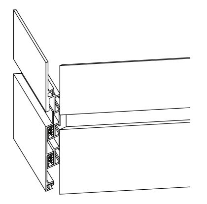
The SLIMLINE alloy baseboards hide into your wall with a minimum height of 58 mm. Any gaps caused by uneven floor installation are sealed with pile brush hidden behide the cover profile.
