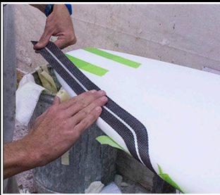
The carbon that runs to the tail acts as a power point under the rear foot and also as a tail patch to minimize pressure denting.
