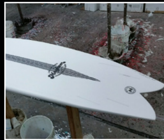
Both the top and bottom feature fused carbon fiber, exo-skeletal stringers
