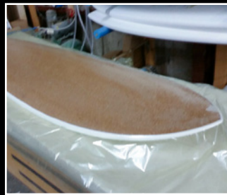
Cork is vacuum bagged to the shaped 1.5lb EPS blank.
