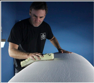
Ultra light, fused cell, EPS blanks provide the core for our unique construction.
