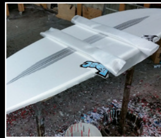
Two layers of 4oz cloth + Fused carbon on bottom.
