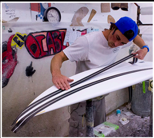
Our carbon fiber bands run the length of the board, creating and controlling our unique torsional flex pattern.
