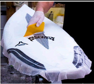
Using optically brightened EPOXY resin, the boards are laminated with a proprietary composite of fiberglass and carbon fiber.
