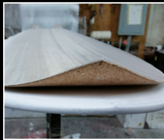
1.5mm cork sandwiched between 60oz fiberglass
