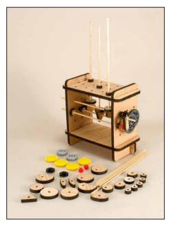
The gear-ratio charts illustrate a variety of gear placements to achieve 1:1, 1:2, 1:2.5, 1:5, and, through a double-reduction gear train, 1:25. One pair of special gears were supplied that enables the user to change the direction of rotation, as with bevel or pinwheel gears. The gears can be placed on their shafts inside the box or outside. The holes in the ends of the box are placed so that appropriately sized gears on adjacent shafts will mesh.
