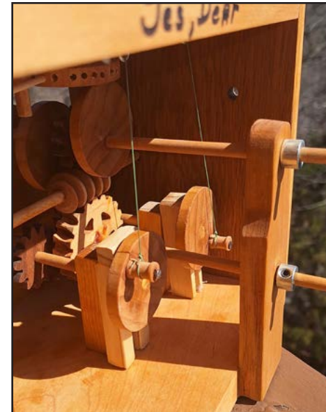
7. Strings are tied to the crankpins on the wooden discs. As the discs revolve, the strings move the man's arms.
