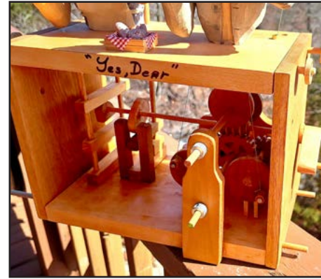
10. The box is held together temporarily during construction by the protruding dowel pegs. Collars with set screws help to locate the various shafts.
