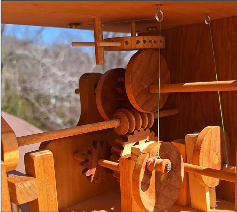
9. This gear train, powered by the worm in the center, operates the man's motions. The two cams above the worm work his head, while the gears below turn the two shafts with the discs, which, through the use of strings, control his arms.
