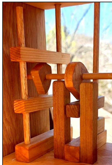
3. The scotch yoke, at the left, with the irregular drive wheel, controls the woman's head, while the eccentric cam at the right raises and lowers her arms.
