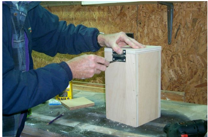
Step 8: Mount the hinge with the screws. Phillips screws are easier to use.
