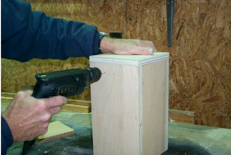
Step 7: Drill small screw starting holes for mounting the hinge.
