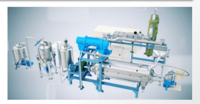
The Celitron ISS AGRI provides a new process to recover solid proteins and oil from Black Soldier Fly larvae, and other edible insects too. The ISS AGRI Facility is a new, unique agriprotein technology, with continuous and automated process system.
