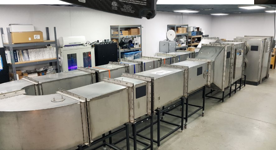
In-house ASHRAE 145.2 Test Chamber
