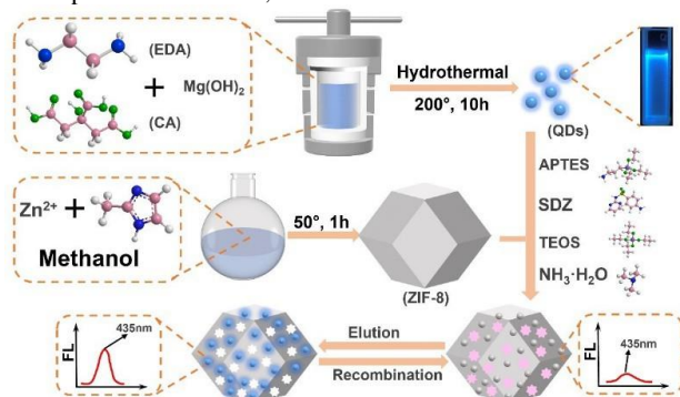
Scheme 1. Synthesis process of \text{SiO}_2@\text{GQDs}@MIPs and its
