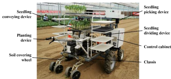
Figure 10. Automatic transplanting machine prototype
