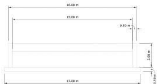
Figure 3: a cross-section of a Balancing Tank
