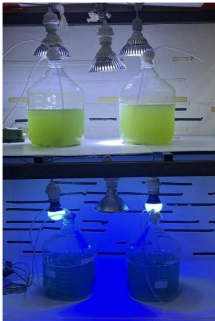
Figure 1 White and Blue LEDs used for the experimental research for study of Phycocyanin content in Spirulina
