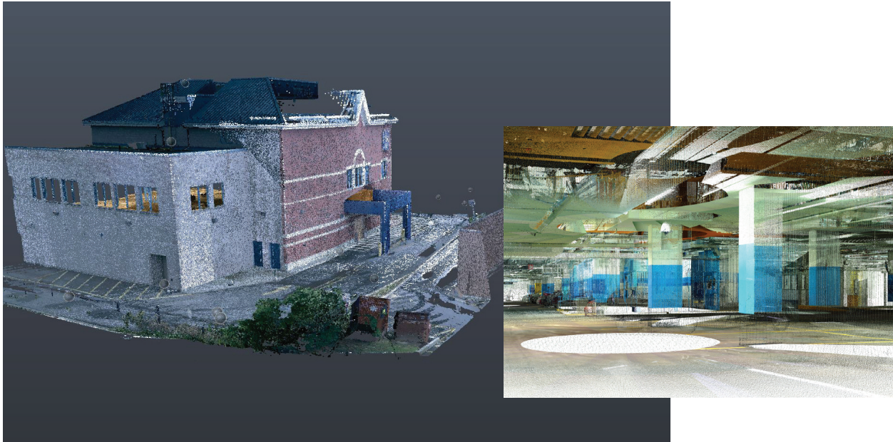
Figure 4 — Point clouds make it possible to quickly generate true-to-life (“as-built”) BIMs in as little time as a few hours
