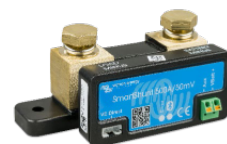
BMV-712 Smart Battery Monitor or SmartShunt enables temperature and voltage compensated charging. The battery charge current information can for example be used to switch from absorption charging to float charging at a set battery tail current.
