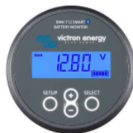
BMV-712 Smart Battery Monitor or SmartShunt enables temperature and voltage compensated charging. The battery charge current information can for example be used to switch from absorption charging to float charging at a set battery tail current.
