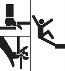
**Liftgate hazards can result in crushing or falling. Keep hands and feet clear of pinch points. If riding liftgate, make sure load is stable and footing is solid.**
