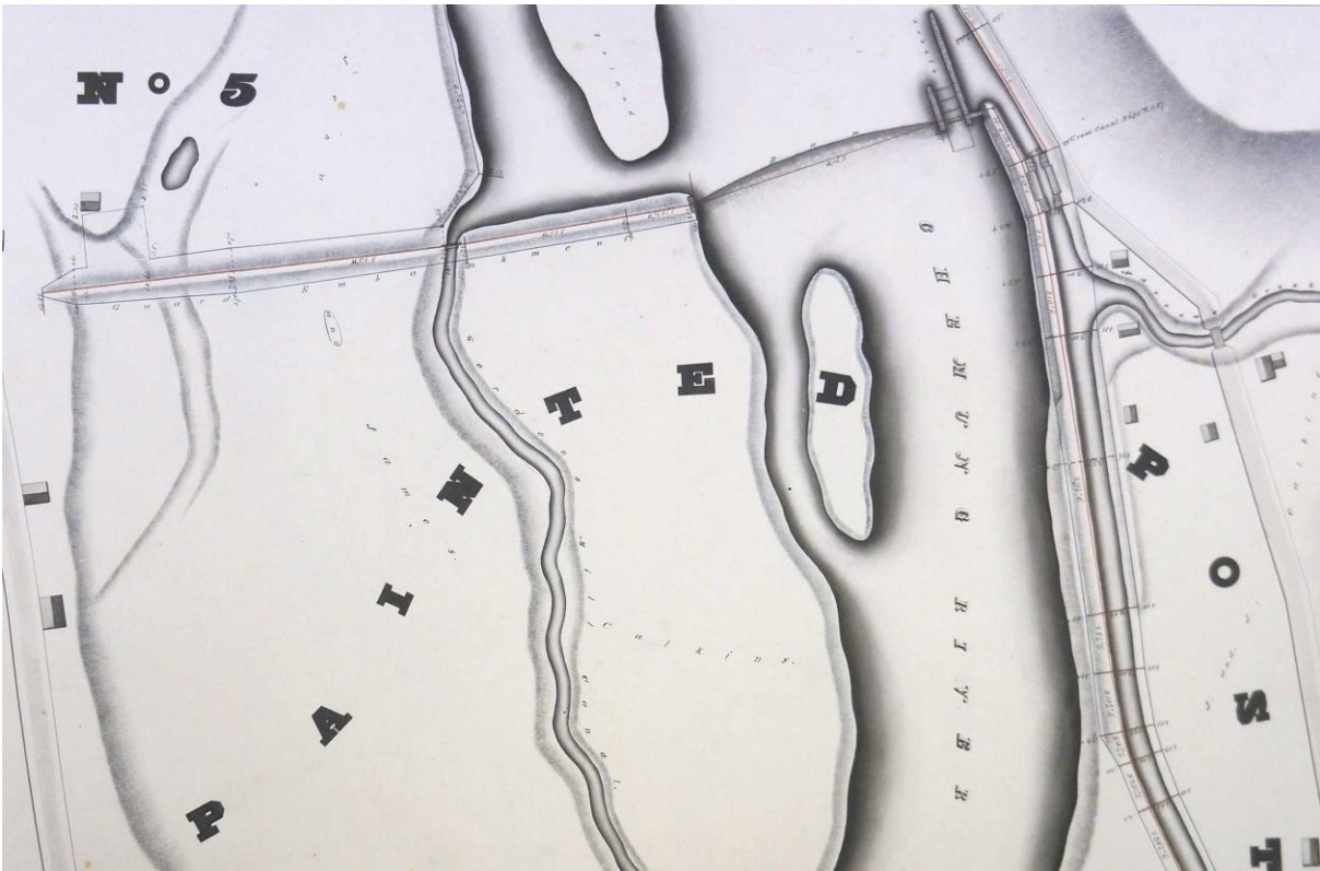
Figure 12. 1843 Holmes Hutchinson Survey of the Chemung Canal, showing feeder dam with canal along right side. Note the narrow channel parallel to the river on the left that fed water-powered mills.
