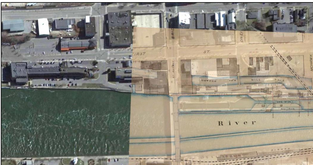
Figures 22, 23, 24. Overlay of c1896 Schillner map onto modern aerial of Oswego Barge Canal Lock 8.
