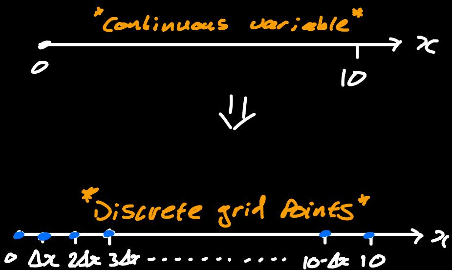
On this discretized  $x$  axis,  $j$  only has a value on the grid points shown.
