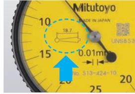
Contact point length is printed on dial face to avoid accuracy issues
