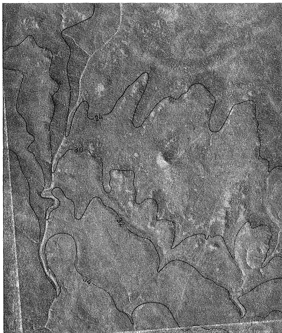
Fig. 4. Limestone, marl and gypsum beds of the lower part of the Tortonian forming questas on the southern slope of the J. Abd El-Aziz. Figures show bed numbers. Here and further on air photograph scale is 1:20,000
