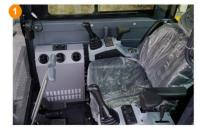
Titan's cab offers a wide, unobstructed sight line in all directions, enhancing safety and awareness on the job site. It can also be equipped with air conditioning, providing a comfortable and operator-friendly working environment.
