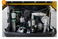
The addition of an air pre-filter enhances filtration efficiency, promoting more complete fuel combustion and improved fuel economy. The flip-up rear engine cover offers streamlined access to internal components, significantly reducing service time and improving maintenance efficiency.
