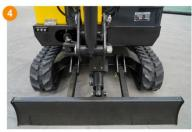
The double-layer Backfill Blades has a longer service life.
