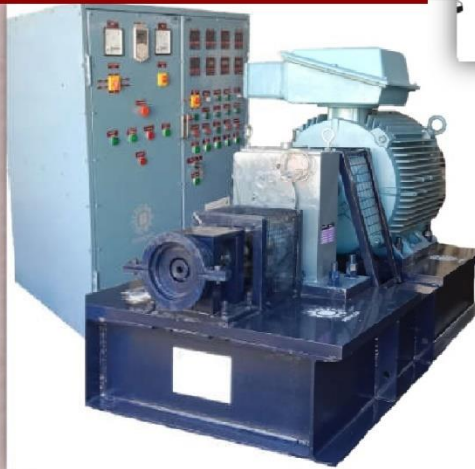
Jaguar Alternator Test Rig - 180HP, 12000 RPM System
