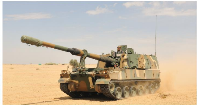
K9 VAJRA-T 155mm / 52 Cal. Tracked Self Propelled Gun
