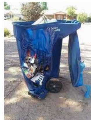
A trash can melted by the blazing Arizona heat
