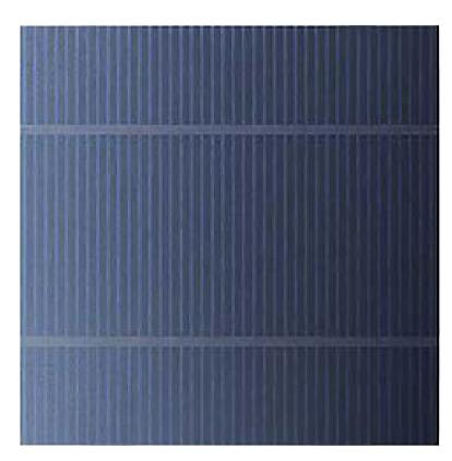
Metal paste is fragile, blocks light and corrodes over time
