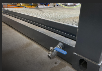
Integrated drip pan with tap allows mobile installation and environmental safety.
