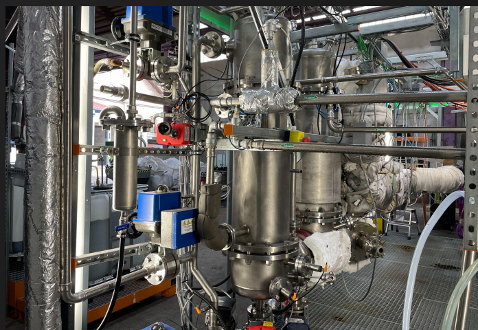
Uninsulated condensers photographed from inside the plant when not in operation.
