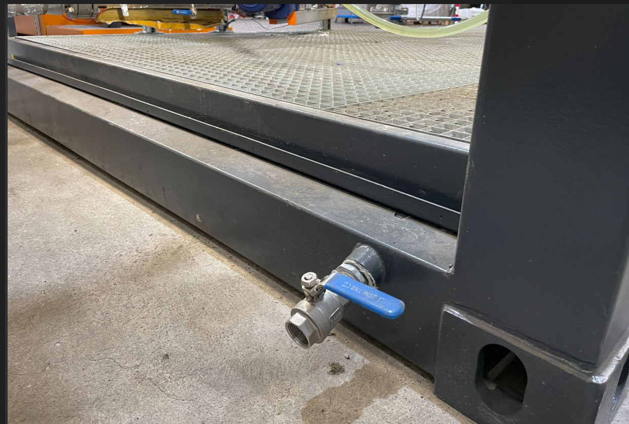
Integrated drip pan with tap allows mobile installation and environmental safety.
