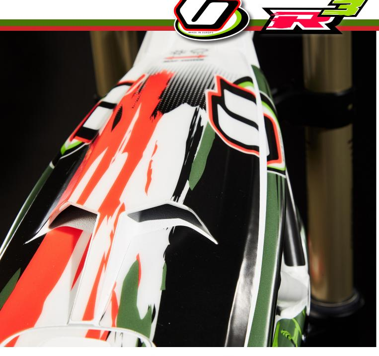
The revised for 2021 airbox helps to greatly increase engine performance. This is thanks to an increased volume and new apertures on the top of the airbox, providing better performance throughout the rev range, especially in lower RPM.
