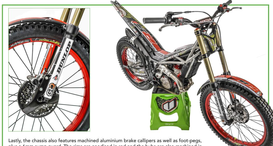
plus a 6mm sump guard. The rims are anodised in red and the hubs are also machined in silver.
