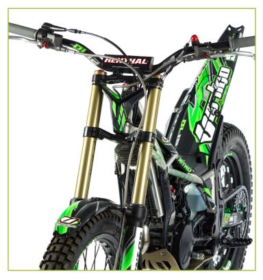
The additional new anti vibration engine support "silent blocks" in the DL12 allows better stability and reduces vibrations.
