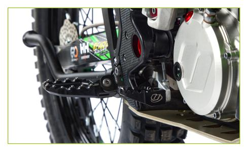
This model also features a re-designed shift selector spring, changing the pre load on the shift selector pulley for more effective gearbox performance, a removable machined clutch cover and the hybrid starting system assisted by battery, to optimise the performance of all electrical components.
