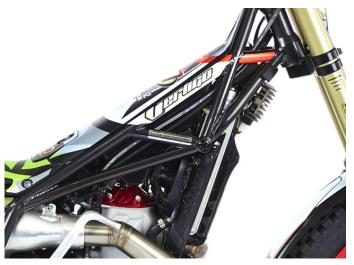
The new for 2020 airbox is a complete new design which helps to greatly increase engine performance. It is also much more rigid and slimmer than the previous model, giving the bike a leaner and more aggressive look. Also new for 2020 is the intercooler which helps keep the engine at it's optimum operating temperature.
