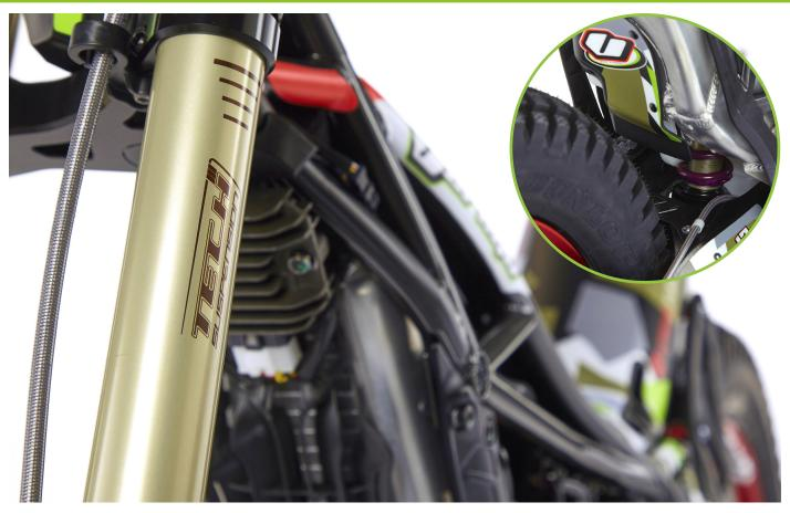
The new Tech Factory spec forks in combination with the multi adjustable 3 way Reiger rear shock provide extremely smooth and responsive feedback to the rider, whilst also allowing any rider to further fine tune their suspension set up depending on their individual riding style.
