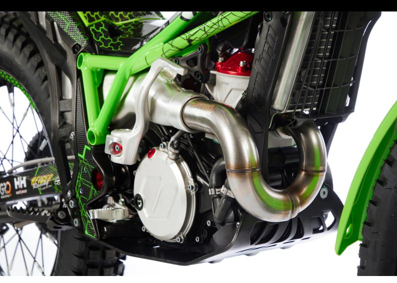
The Nitro 2023 incorporates a detachable two-piece clutch cover as standard feature, one of Vertigo's great advances from last year in its top models, and a unique engineering piece of work that adds exclusivity and style, while also facilitates maintenance tasks.
