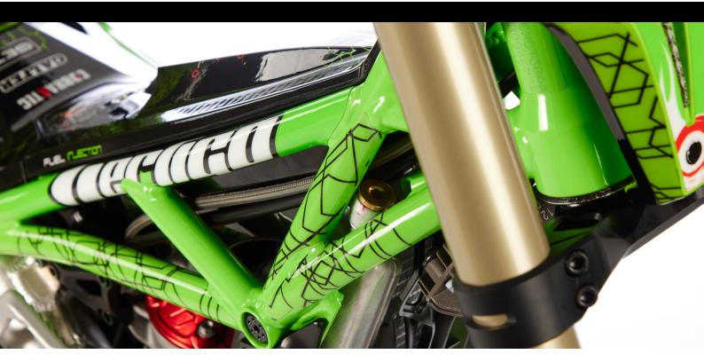
The known maneuverability and dynamics of Vertigo's revolutionary steel frame is matched by the 170mm Tech Factory fork and the Reiger 2-way shock absorber anchored by micro-casting, adjustable in compression, rebound and preload, achieving a stable and responsive motorcycle.
