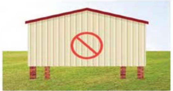
No Installs on Stacked Blocks
