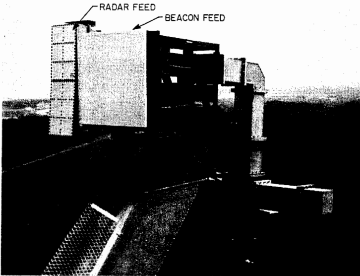
FIG. 33-15 Integral beacon feed for the ARSR-3. (Courtesy Westinghouse Electric Corp.)
