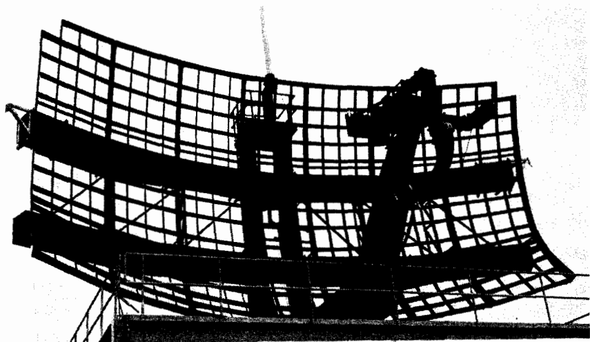
FIG. 32-2 ARSR-3 2D antenna. (Courtesy of Westinghouse Electric Corp.)
