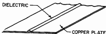
FIG. 42-24 Image line using HE_{11} mode.
