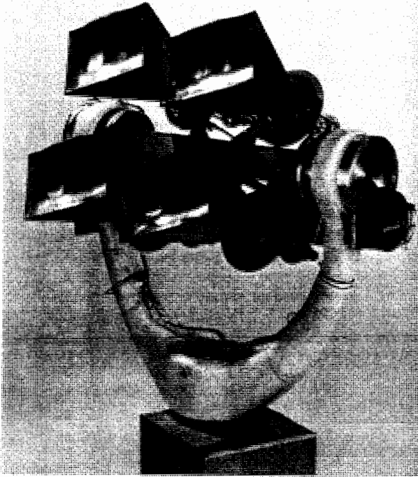
FIG. 40-7a Four-horn sequential-lobing tracking antenna (1 to 5 GHz).
