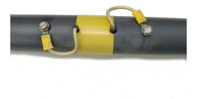
The picture below illustrates the correct placement of the GAP TITAN Guy clamp. This clamp should be placed immediately above the "GAP". Take care when attaching your guy ropes to ensure they do not contact the tuner rods as this will cause wear and eventual failure of the guy ropes from motion.
