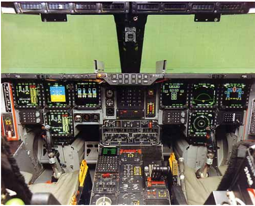
The B-2 (cockpit) was the first aircraft equipped with color, nine-tube, electronic flight instrument systems and multi-purpose panels for displaying flight, engine, and sensor data, and avionics systems and weapons status. (USAF)
