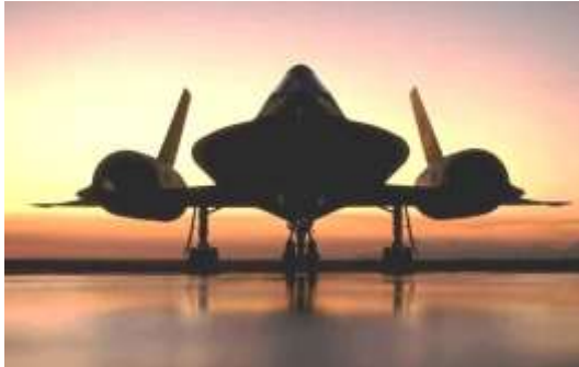
Lockheed SR-71 Blackbird was the first stealth-design aircraft designed for strategic military reconnaissance, designed with a wingspan of 55'7", speeds of Mach 3.2, and altitudes of 85,000+. (Photo courtesy: Lockheed Martin.)
