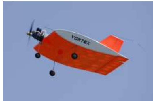
The Tucker Vortex is a blended body invention designed not to stall. (Photo Courtesy: Chuck Tucker.)
