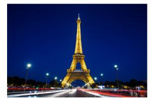
If you want to see the Eiffel Tower in all of its glory, then you might want to head to Paris in the summer. That's because the 1,062-foot monument is more than six inches taller in the heat, thanks to thermal expansion, which causes the iron structure to expand, according to the *Los Angeles Times*. Even crazier, once the sun sets the tower begins to shrink again.
