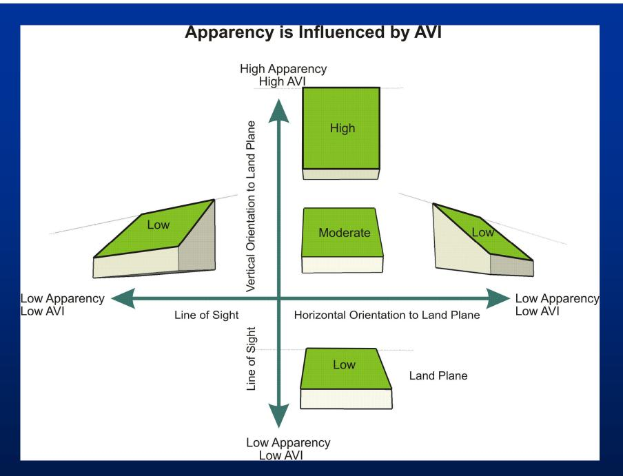
Angle of Visual Incidence (AVI) is *the angle between the sight line and the land plane at the point of incidence*.
