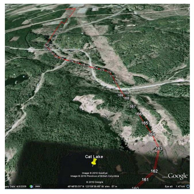
Figure 4. VQA Segment 3 looking west from Polepoint 160 where the proposed line travels parallel to the existing 500 kV BC Hydro line 5L045 and 230 kV BC Hydro line 2L002 past Cat Lake, crossing Highway 99, then parallels the existing small transmission line, crossing Highway 99 twice again before reaching the Cheekye substation (top of picture).
