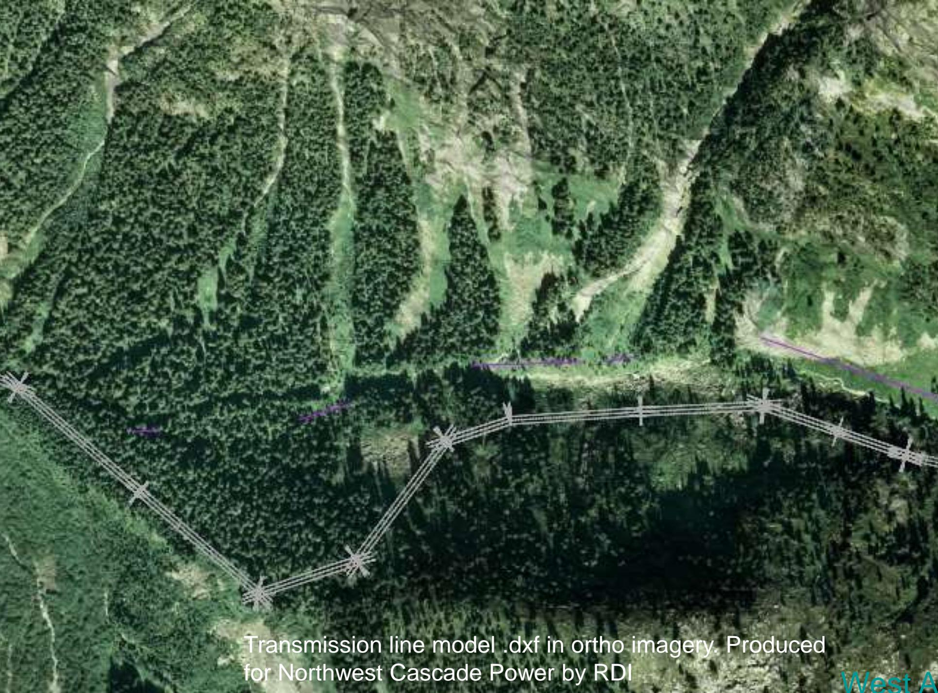
Transmission line model .dxf in ortho imagery. Produced for Northwest Cascade Power by RDI
