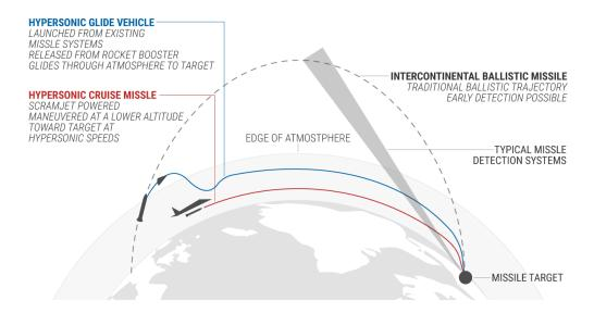
Figure -1: Illustration highlighting the issues with response time compression due to the point of detection of a hypersonic missile <sup>20</sup>.
