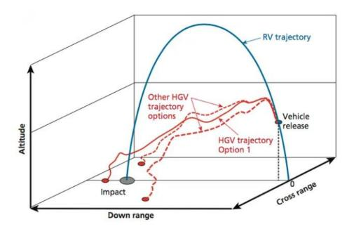
Figure-2: Illustration of ballistic re-entry vehicle (RV) compared to the trajectory of a hypersonic glide vehicle <sup>24</sup>.
