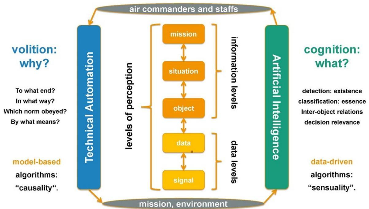
Figure 4. Levels of AI-assisted perception and action for command and control, ISR, engagement, and impact assessment. © Fraunhofer FKIE.
