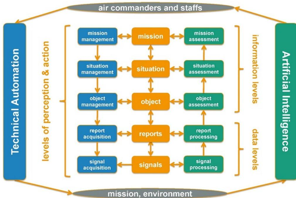
Figure 5. Map of the algorithms that drive artificially intelligent automation in AirC2 with inter-related OODA loops on every level. © Fraunhofer FKIE.
