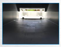
Avoid expensive floor repairs. Our single piece floor and hopper components are made of Hardox 450 steel which is 5 times more abrasion resistant than mild steel.
