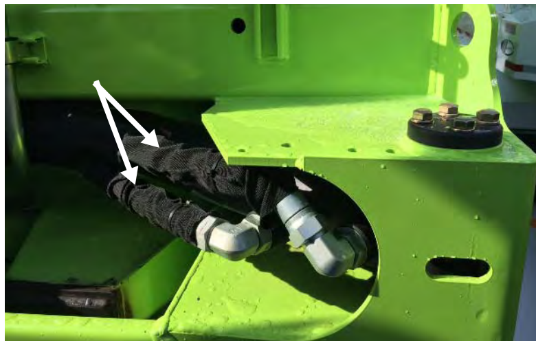
Figure 3-34 Location of cylinder hydraulic hoses
