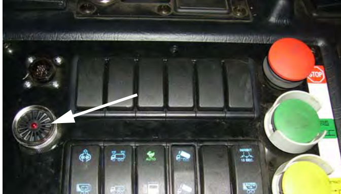
Figure 9-18 Buzzer with red light in its center
