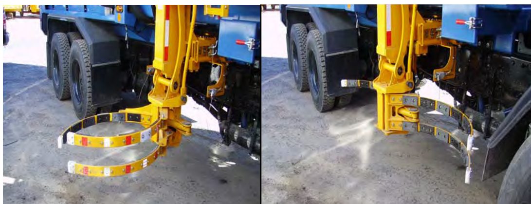
Figure 10-8 Gripper closed (left) and open (right)
