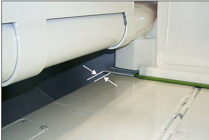
Figure 3-80 Packer at about one inch from fully extended position
