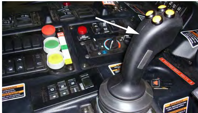
Figure 9-20 CAN bus-based multiplex joystick
