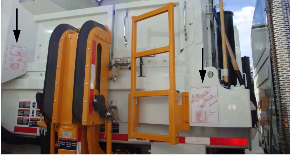
Figure 4-10 Lube charts on vehicle right-hand side
