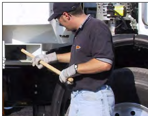
Figure 3-6 Removing debris through the clean-out trap
