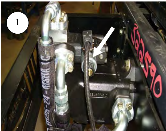
Figure 5-1 Vane pump solenoid valve on the pump (1) and on the chassis (2)
