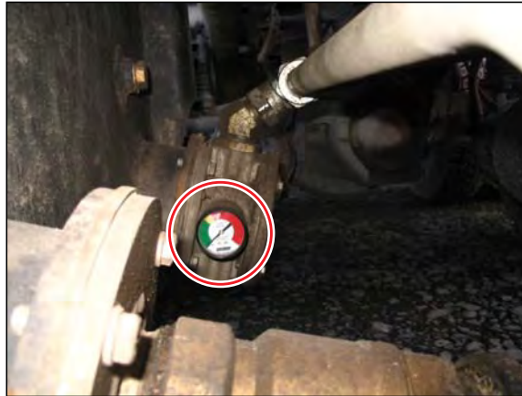
Figure 5-34 Filter restriction indicator (steel tank)
