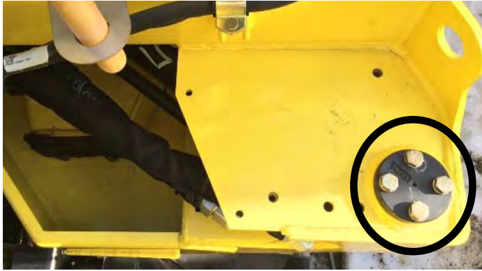
Figure 3-35 Bolts securing piston side of cylinder
