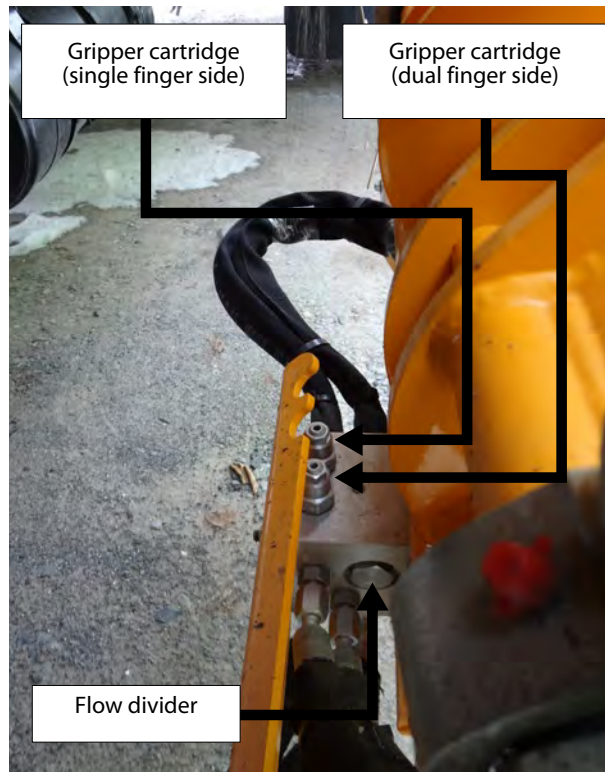
Figure 10-15 96-gal gripper holding valve
