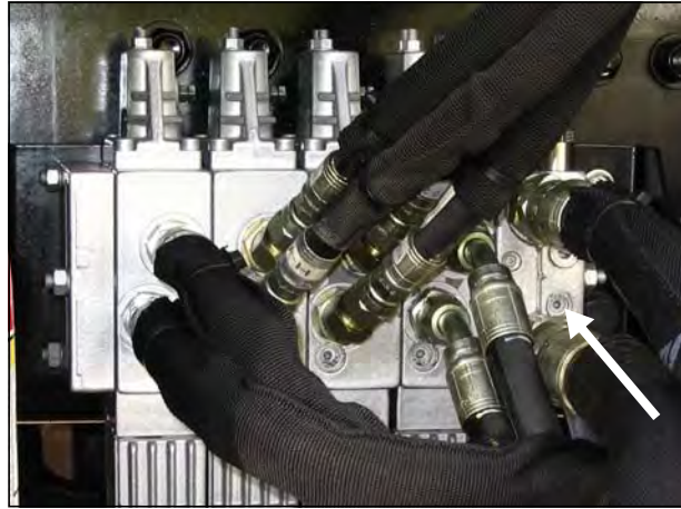
Figure 5-23 Main relief valve adjustment screw
