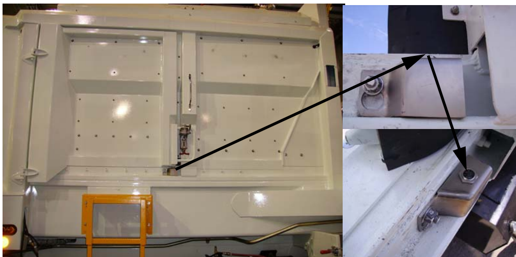
Figure 2-57 Hopper Door Proximity Switch
