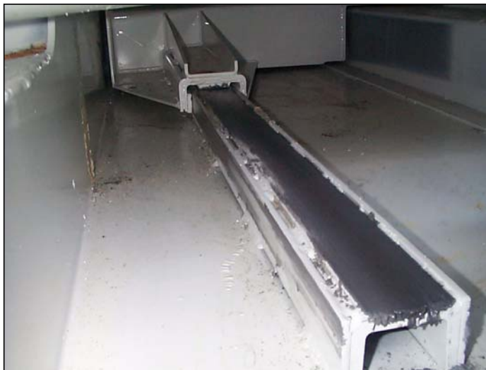
Figure 2-27 Packer sitting on the floor guide
