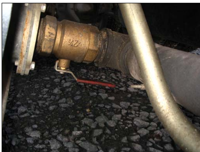
Figure 1-12 Suction line mounted valve (steel tank)
