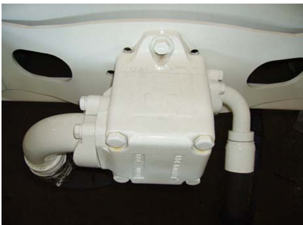
Figure 4-1 Vane pump (left) and solenoid valve on the chassis (right)
