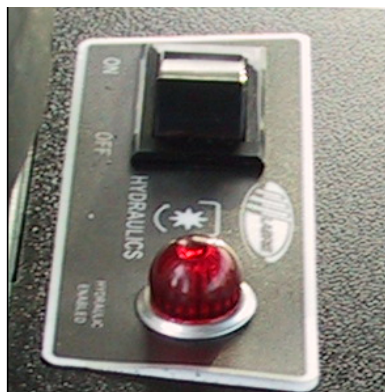
Figure 1-11 Hydraulic pump ON/OFF switch and indicator light
