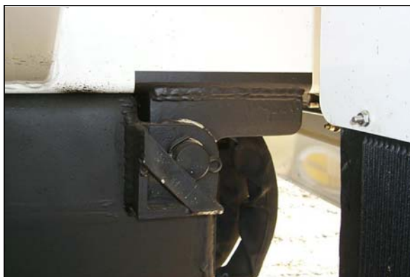
Figure 3-18 Body hinge (view from behind the rear mudguard)
