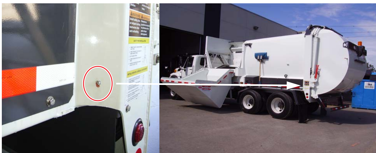
Figure 3-22 Location of the remote grease fitting (near tailgate)
