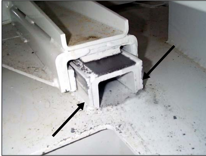
Figure 2-30 Welds on both sides of the floor guide
