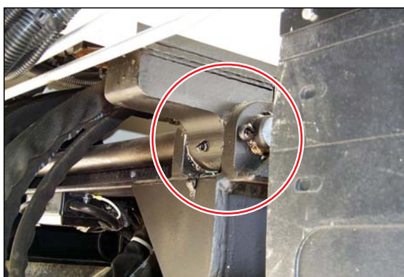
Figure 3-18 Body hinge (view from behind the rear mudguard)
