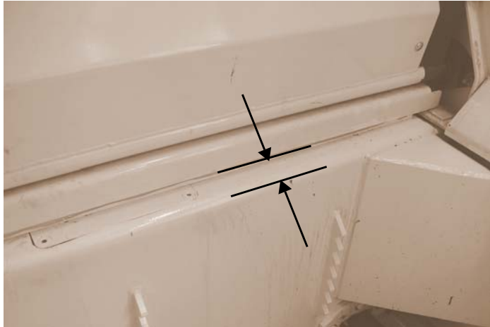
Figure 2-51 Packer retracted about one inch before end of stroke
