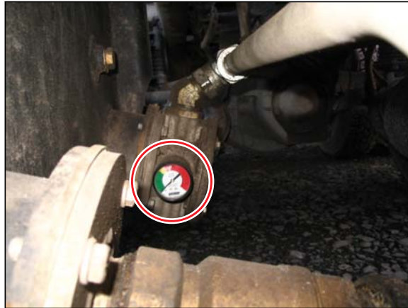
Figure 4-17 Filter restriction indicator (steel tank)
