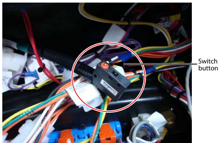
Figure 7-4 The multi-cycle configuration switch
