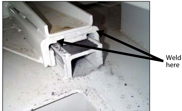
Figure 2-20 View from behind the packer (packer fully retracted)
