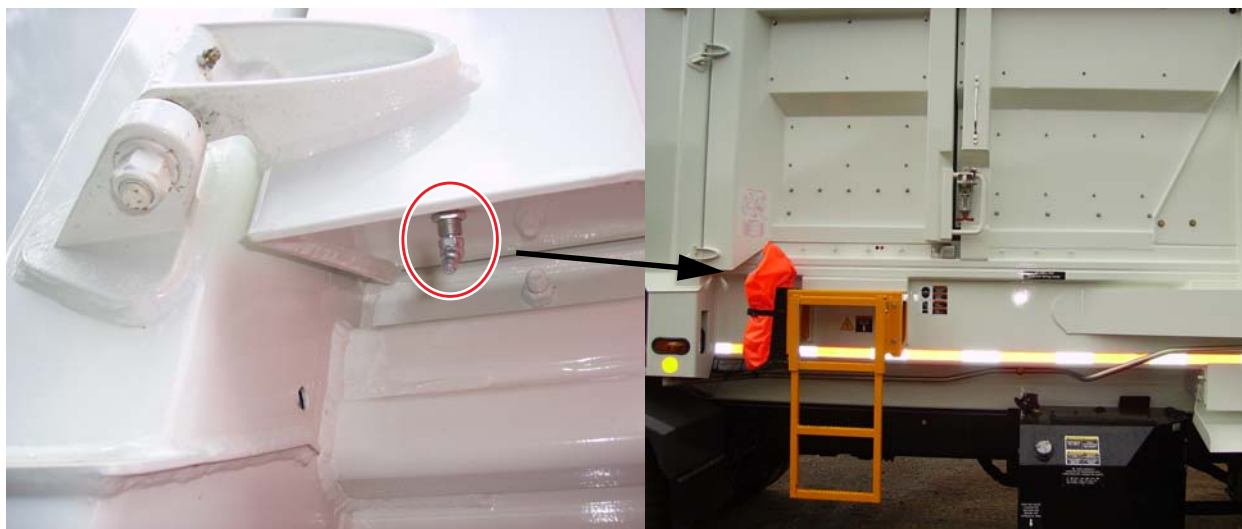
Figure 3-23 Location of the remote grease fitting (hopper door)
