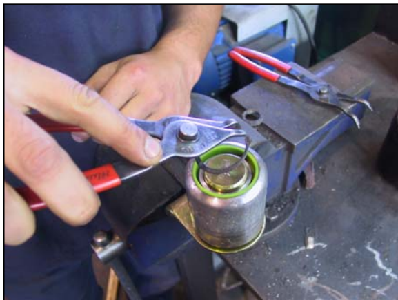
Figure 2-33 Removing the external snap ring
