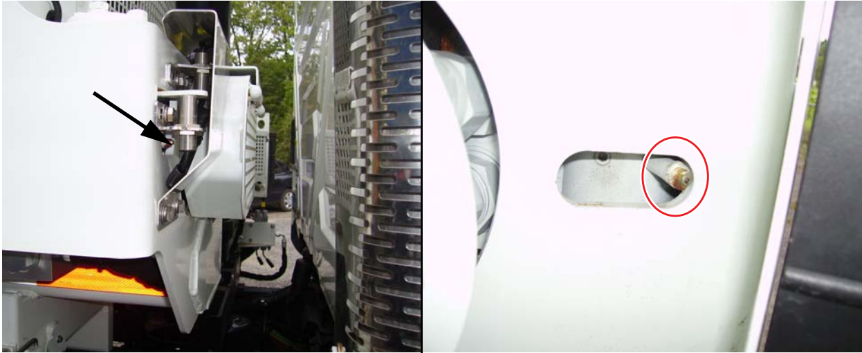
Figure 3-24 Location of the grease fittings (curbside, left; street side, right)
