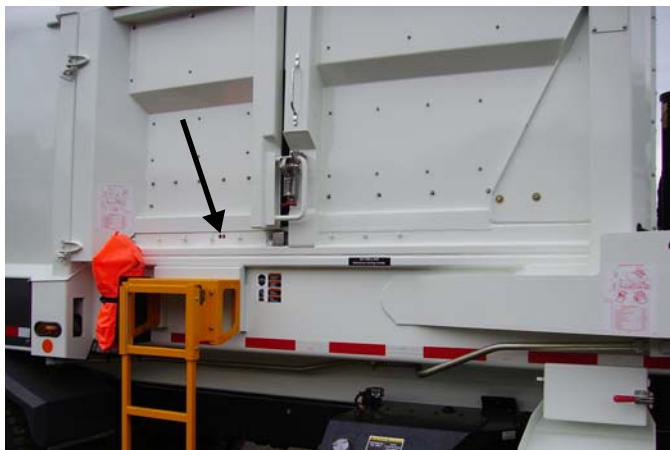
Figure 3-25 Location of the hole allowing access to the remote grease fitting
