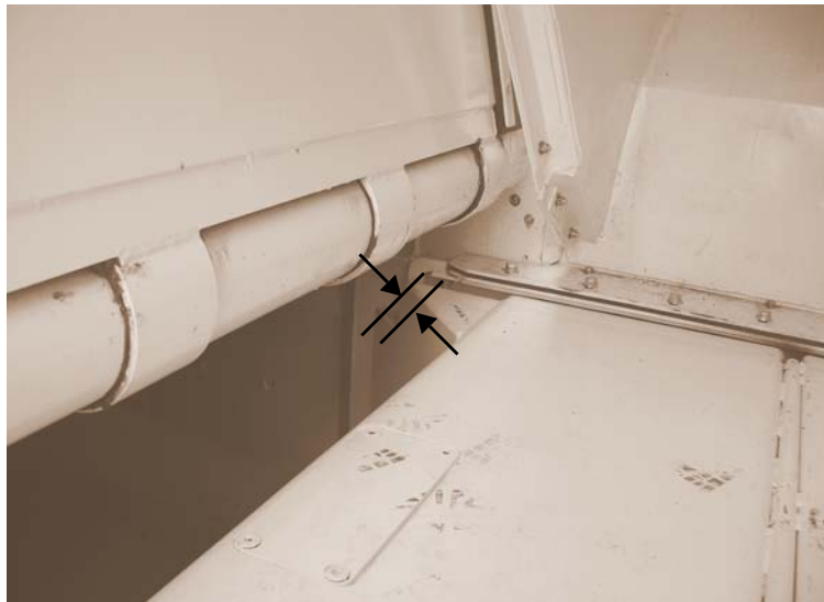
Figure 2-48 Packer extended back by about one inch
