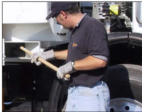
Figure 2-7 Removing debris through the clean-out trap
