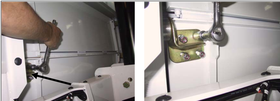
Figure 2-32 Removing the four bolts
