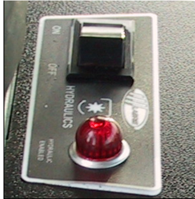
Figure 2-10 Hydraulic pump ON/OFF switch and indicator light
