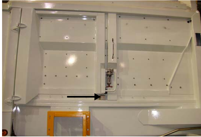
Figure 4-18 Hopper Door Proximity Switch
