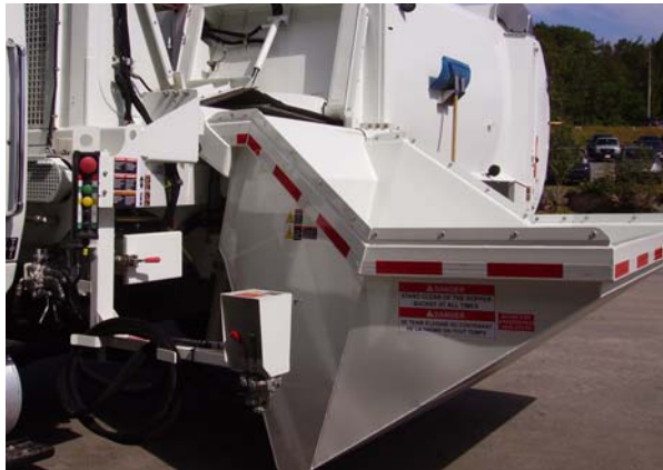
Figure 4-21 Unfold swivel arm and bucket down
