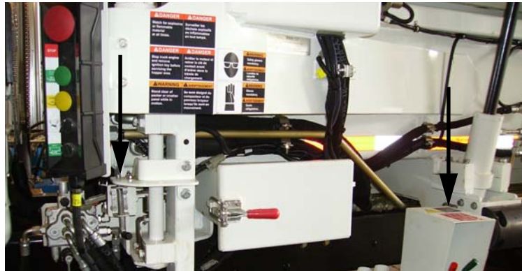
Figure 4-15 Position of the arm lock levers
