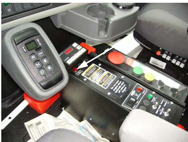
Figure 3-3 TAILGATE UNLOCKED or BODY RAISED warning lamp
