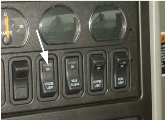
Figure 3-10 Strobe light switch (left); strobe light (right)
