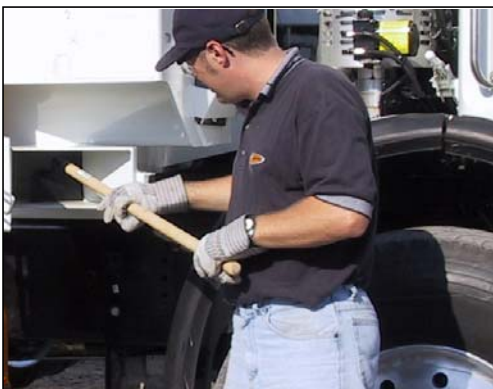
Figure 2-12 Removing debris through the clean-out trap
