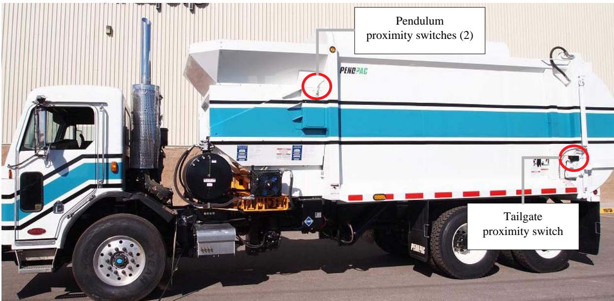
Figure 3-22 Location of the proximity switches (streetside)
