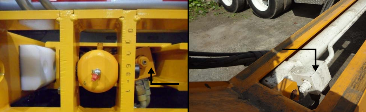
Figure 3-46 Streetside holding valve (left) / Curbside holding valve (right)
