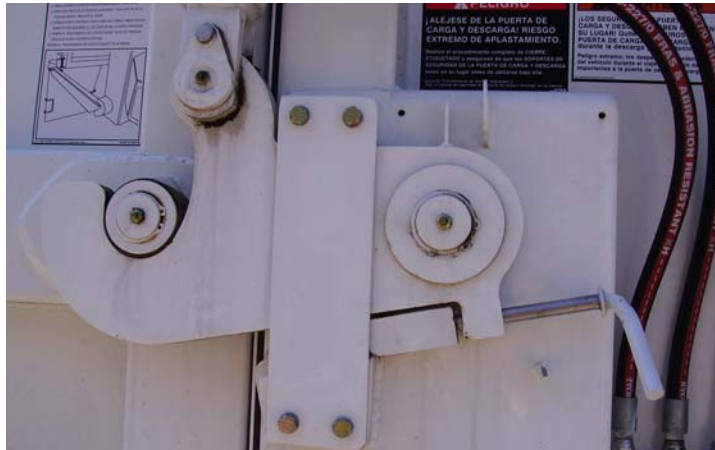
Figure 2-10 Tailgate safety lock in removed position
