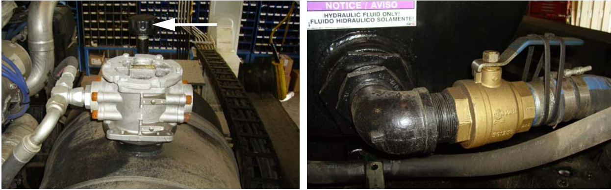
Figure 3-3 Breather cap, left / ball valve, right
