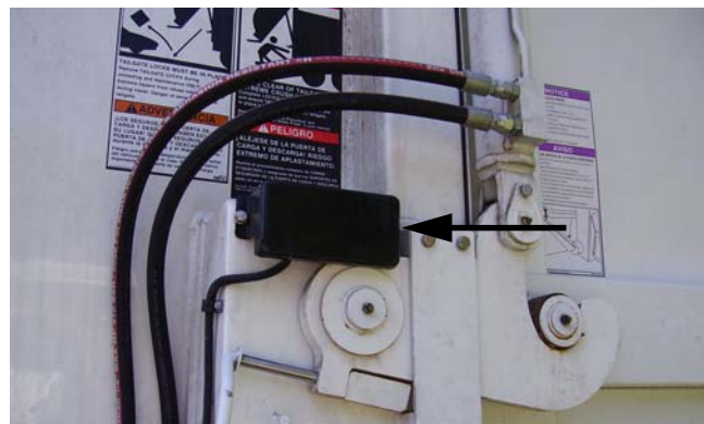
Figure 3-31 Cover protecting the tailgate open proximity switch
