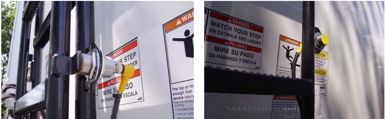
Figure 3-23 Access ladder proximity switch: ladder in “home” position, left; ladder in deployed position, right
