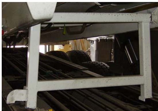
Figure 2-23 Hoist safety prop in engaged position
