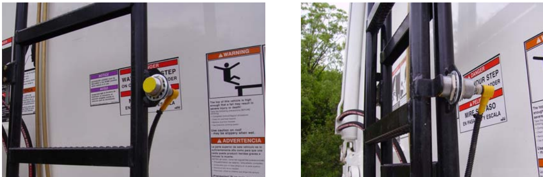
Figure 2-3 Extension ladder proximity switch with ladder deployed (left) and in stored position (right)
