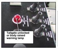
When the body is raised, the Tailgate unlocked or body raised warning lamp turns on and a buzzer sounds.
