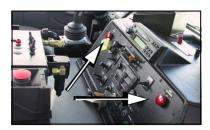
Two warning lights on the dashboard indicate to the operator when the arm is out. Do not move the vehicle until these lights stop flashing.
