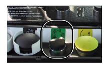
This optional function allows the packer to cycle a preset number of cycles (from 2 to 8, 3 being the standard) by pressing the green button once. Cycles can be stopped anytime by pressing the red button or if the multi-cycle control button is turned off.
