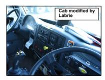
If the cab of the vehicle has been modified by Labrie Environmental Group (right-hand side driving position) for door-to-door waste collection, the maximum speed limit while driving at the right-hand side is, if permitted, 20 mph. (32 km/h). Therefore, it is recommended to drive on the left-hand side for any long distance driving (if the truck is equipped with a left-hand side driving position).
