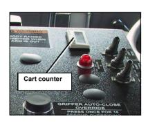
Some units are equipped with a cart counter, which counts the number of carts dumped. The counter (if equipped) is located on the cab console.
