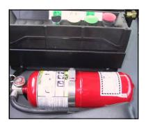
The fire extinguisher provided is 5 lbs (minimum capacity). It must be checked regularly by qualified personnel.
