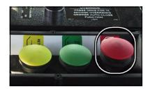
The Emergency Stop button (red) will stop all hydraulic functions on the truck (tailgate, arm etc.). By pressing the red button, the packer and the arm will stop where they stand. The red button has to be manually pulled back to reactivate the hydraulic system.
