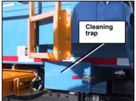
Clean all the truck's lights and safety stickers, so you and the surrounding pedestrians and vehicles will be aware of the truck at all times. Use the hoe to rake dirt out of cleaning traps on each side of the vehicle.
