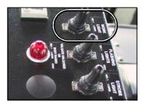
When installed, this switch activates and deactivates the work lights.
