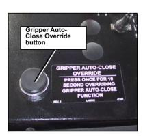
The Gripper (or grabber) Auto-Close Override function (standard) allows the operator to open the grabber in the hopper in order to throw away the grabbed object directly in it. It also allows to pick up elevated carts.
