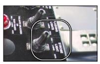
This switch activates and deactivates the strobe light mounted on the tailgate.
