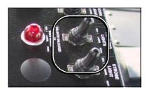
This switch activates and deactivates the strobe light mounted on the tailgate.
