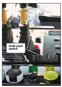
The grab pack switch enables the packer to automatically start cycling about 4 seconds after the grabber is closed. This gives the arm enough time to reach the hopper and dump the cart before the packer starts to pack.
