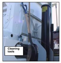
Daily cleaning of the hopper and chassis is crucial because it will minimize breakdowns and maintenance expenses. Daily wiping down of all truck lights, warning lights and safety stickers will make your vehicle more visible so that surrounding pedestrians and vehicles will be safer around the vehicle.
