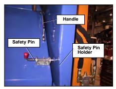
Figure 49. Swivel-style panel safety devices
