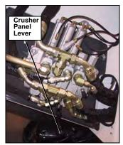
Figure 123. Crusher panel lever
