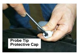
Figure 188. Sample bottle probe tip
