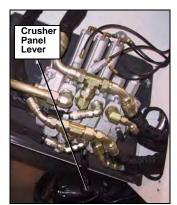
Figure 36. Crusher panel lever
