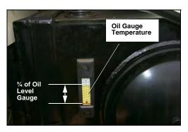
Figure 143. Hydraulic Tank Gauge
