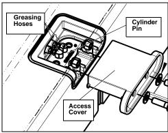
Figure 104. Packer cylinder pins, access cover and greasing hoses
