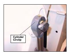
Figure 129. Tailgate left cylinder circlip
