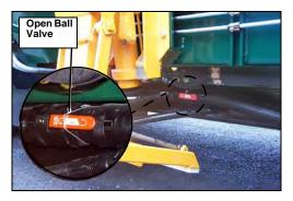
Figure 29. Suction-line-mounted valve
