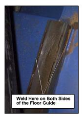
Figure 109. Floor guide top-view
