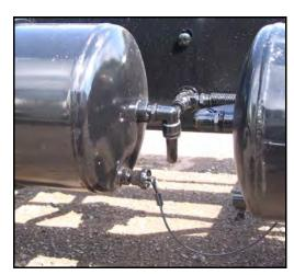
Figure 31. Air tank with steel cable on drain valve
