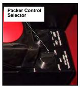
Figure 95. Packer control selector switch
