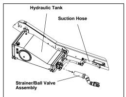
Figure 151. Strainer removal
