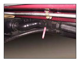
Figure 170. Ball valve in closed position
