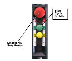
Figure 65. Right-hand side control station
