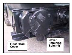
Figure 147. Hydraulic tank's filter head cover
