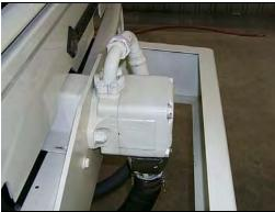
Figure 155. Vane pump
