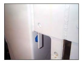
Figure 141. Proximity switch front-view
