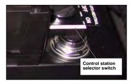
Figure 22. Control station selector switch
