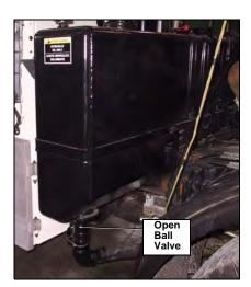
Figure 28. Main hydraulic tank ("saddle" model)
