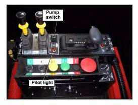
Figure 13. Pump switch and pilot light on the console
