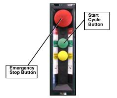
Figure 37. Right-hand side control station
