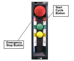
Figure 124. Right-hand side control station
