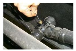
Figure 185. Pressing the coupler spring ball
