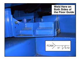
Figure 110. Floor guide end-view
