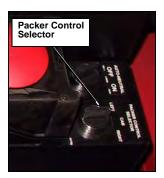
Figure 117. Packer control selector switch
