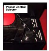
Figure 86. Packer control selector switch
