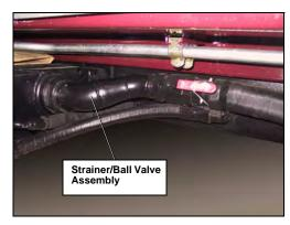
Figure 153. Strainer/Ball Valve Assembly
