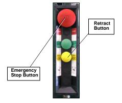
Figure 98. Right-hand side control station
