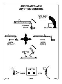
Figure 12. Helping Hand™ joystick functions
