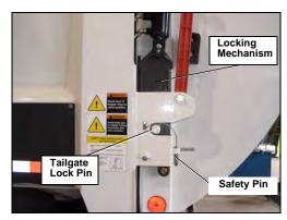
Figure 131. Tailgate locking components
