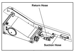
Figure 154. Strainer removal
