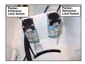
Figure 66. Packer cylinder limit switches
