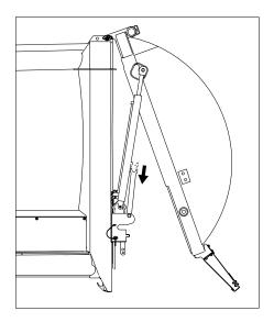
Figure 10. Putting the tailgate safety prop back in its home position
