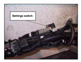
Figure 64. Multi-cycle settings switch
