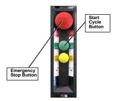
Figure 71. Right-hand side control station
