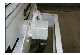
Figure 169. Hydraulic pump on front bumper
