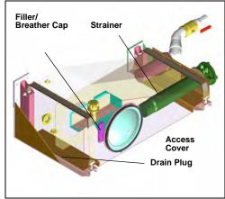
Figure 149. Hydraulic tank
