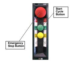
Figure 118. Right-hand side control station
