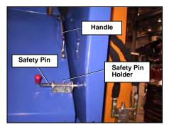
Figure 114. Swivel-style panel safety devices
