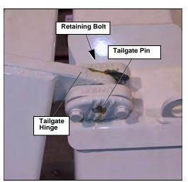
Figure 130. Right side tailgate hinge and pin
