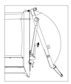
Figure 7. Pulling the tailgate safety prop out from its home position
