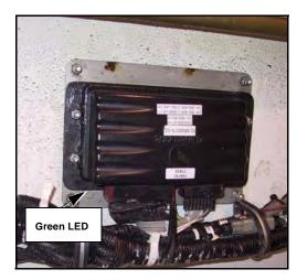
Figure 62. Packer multi-cycle module
