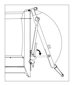
Figure 8. Putting the tailgate safety prop in its set position
