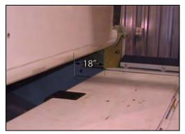
Figure 81. Packer extended 18" from end of stroke
