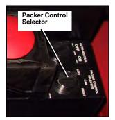
Figure 67. Packer control selector switch
