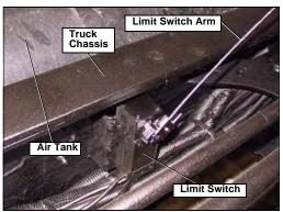
Figure 138. Body raised limit switch
