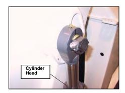
Figure 133. Right-hand side tailgate cylinder
