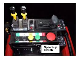
Figure 20. Speed-up switch
