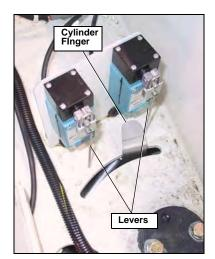
Figure 127. Packer cylinder limit switches
