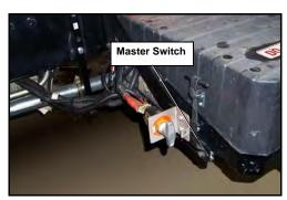
Figure 3. Master switch location
