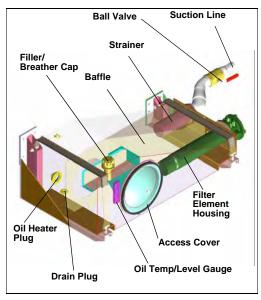
Figure 144. Hydraulic Tank
