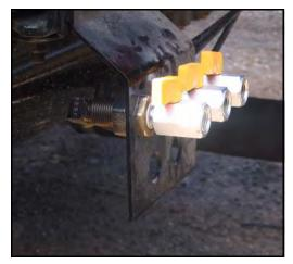
Figure 32. Ball valves with extension hoses
