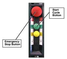
Figure 58. Right-hand side control station
