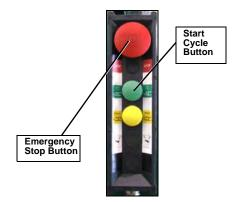
Figure 44. Right-hand side control station
