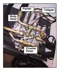
Figure 142. Main hydraulic valve
