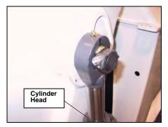
Figure 128. Right-hand side tailgate cylinder
