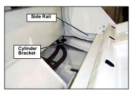
Figure 51. Cylinder bracket and side rails (left-side view)
