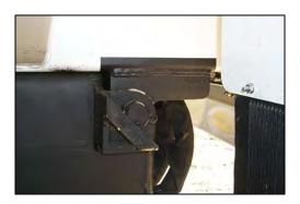
Figure 137. Body-to-chassis left hinge
