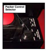
Figure 33. Packer control selector switch
