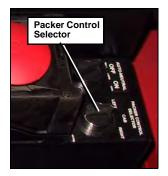
Figure 54. Packer control selector switch
