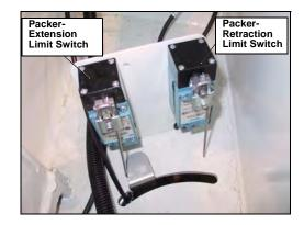
Figure 73. Packer cylinder limit switches
