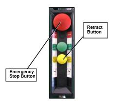
Figure 89. Right-hand side control station
