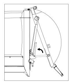
Figure 9. Raising the tailgate safety prop upward
