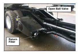
Figure 27. Main hydraulic tank (pressurized model)
