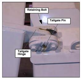
Figure 134. Right side tailgate hinge and pin
