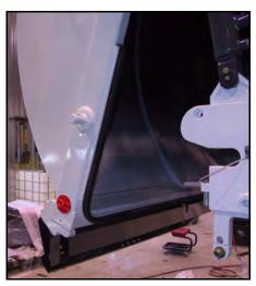
Figure 132. Tailgate rubber seal
