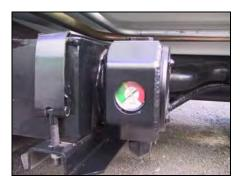
Figure 146. Filter restriction indicator
