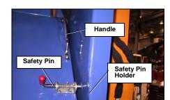
Figure 53. Swivel-style panel safety devices
