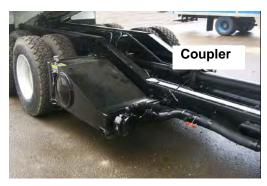
Figure 182. Standard hydraulic tank
