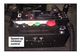
Figure 21. Speed-up inhibitor control
