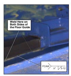
Figure 111. Floor guide end-view
