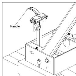
Figure 5. Safety prop release handle
