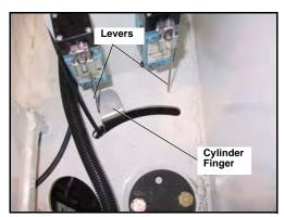
Figure 76. Packer limit switches
