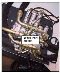
Figure 164. Main hydraulic valve
