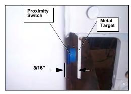
Figure 140. Proximity switch side-view
