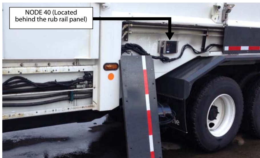
Figure 3-21 Node 40 module location
