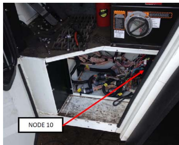
Figure 4-1 Example of a Mack chassis node 10 installation
