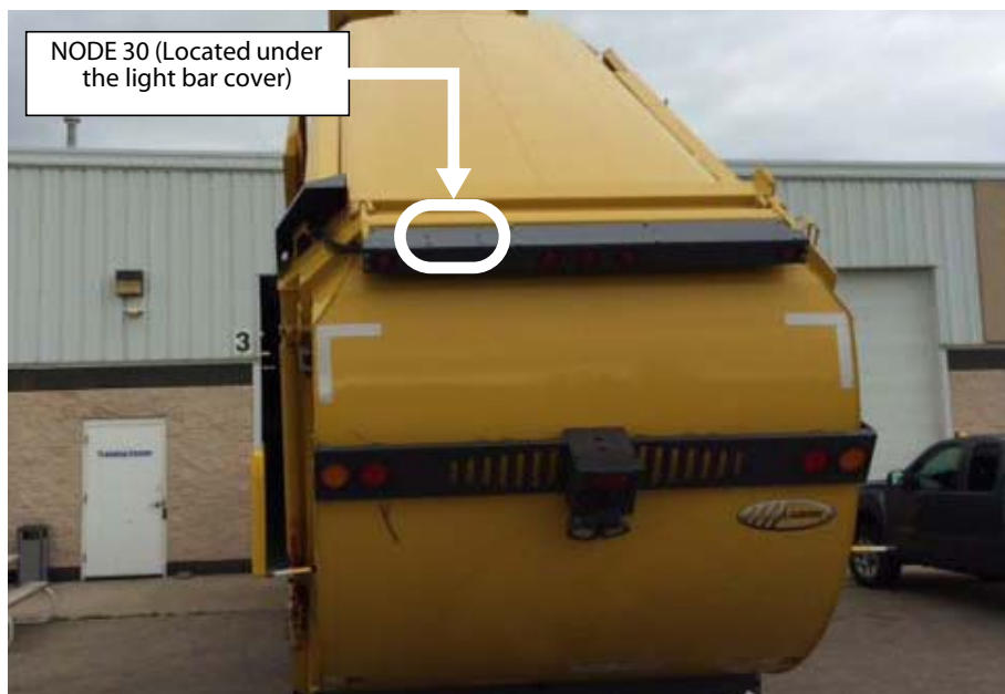
Figure 3-20 Node 30 module location
