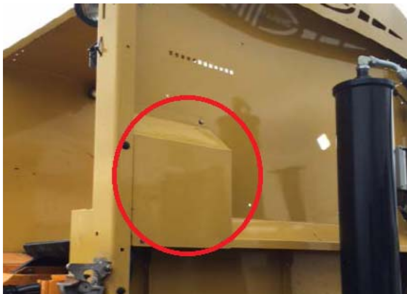
Figure 3-22 Node 50/60 module location
