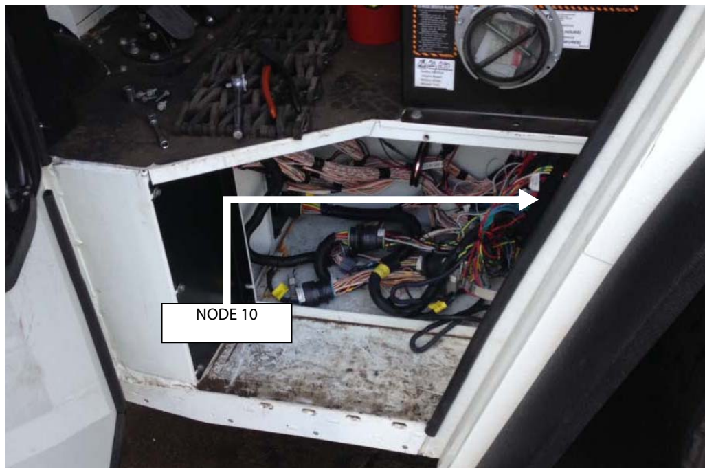
Figure 3-18 Module location on a Mack LEU chassis
